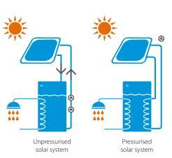
for heating and domestic hot water. The solar unit uses an advanced lightweight plastic tank incorporating exceptional hygienic properties to protect against contamination. In case of an unpressurised solar system our flow-through design, prevents bacteria cannot become to establish and grow. This eliminates the need for a thermal disinfectant cycle.
